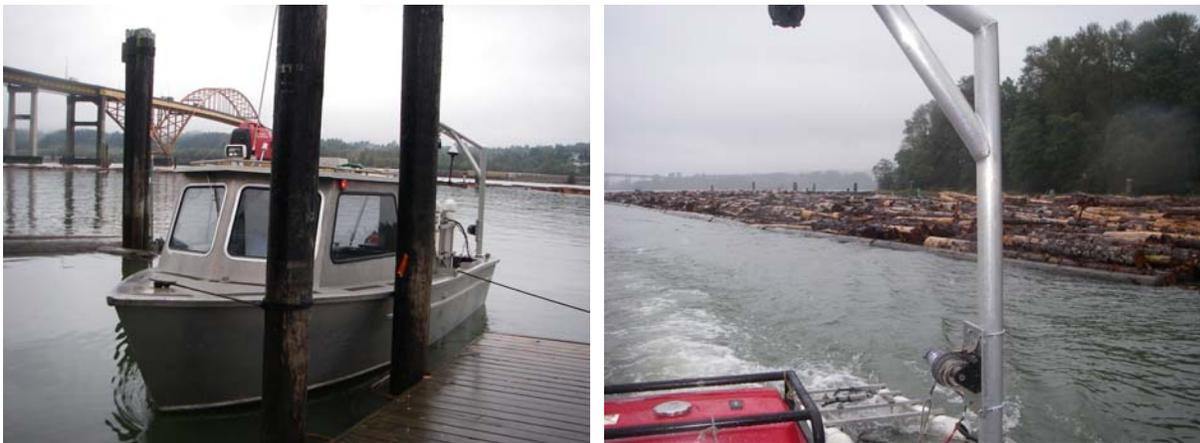
Figure : Terra Remote Sensing Inc. research vessel that is used as the operating platform for seismic profiling docked on the left photograph and operating the boomer system (center bottom of picture) on the right photograph.
