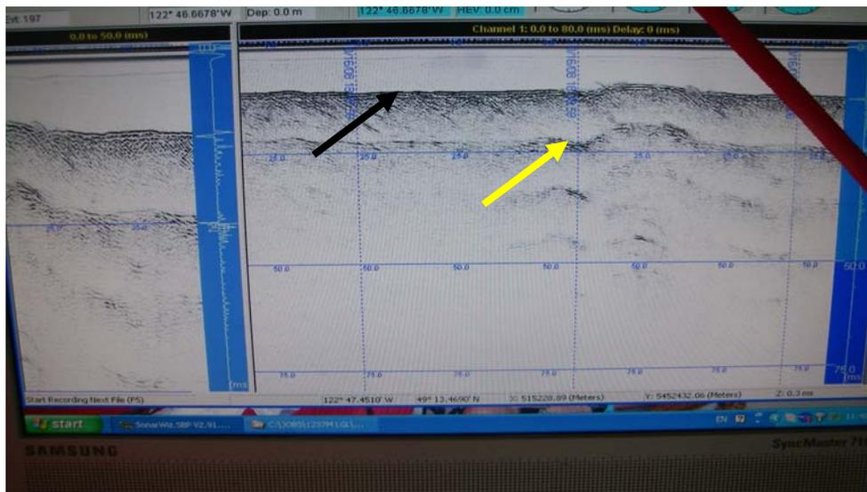
Figure : Typical printout and hardcopy back-up from seismic sub-bottom profiling showing river bottom (black arrow) and the first layer of substrate with different physical features (yellow arrow). The soft layer
